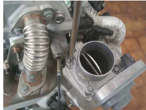
B Loosen the 4 screws with an 8 mm wrench
