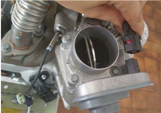
A Disconnect the plug
